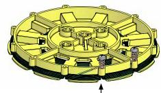
The arrows show the direction to coil the wire around each stator. Notice that every other coil is wound in the opposite direction.
