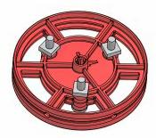
Loosely attach two wheel hubs, as shown, using #10 x 1 inch machine screws and nuts.
